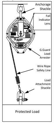
In the event of a fall, rope is pulled out of the unit at an accelerating rate. On reaching the activation speed the braking mechanism will engage. The energy of the fall is dissipated and the load brought to a halt. There should be adequate clearance below the protected load to safely stop a fall.
